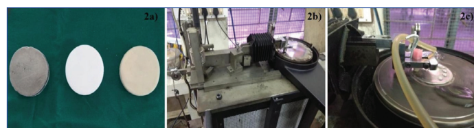
[Table/Fig-2]: a) Disc specimens made of metal, zirconia, and metal-ceramic materials, each measuring 60 mm in diameter and 10 mm in thickness; b) Pin on disc testing machine; c) Distilled water irrigated during testing.
